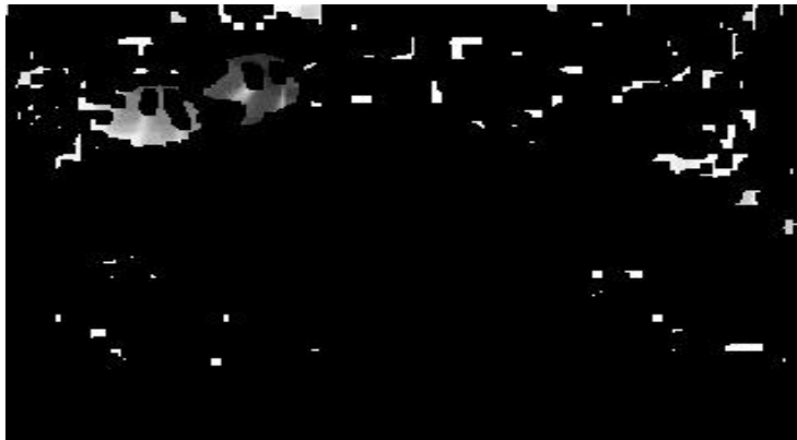
Fig. 3. An example mask computed by background subtraction and erosion indicates the region of background
