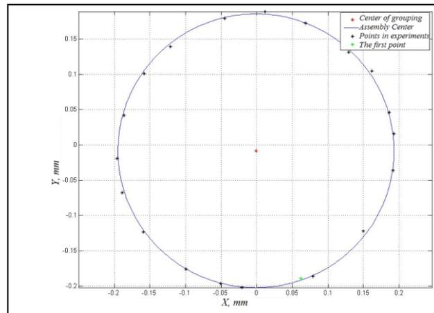
Fig. 2. A graphical solution for finding the center of mating and outrun.
