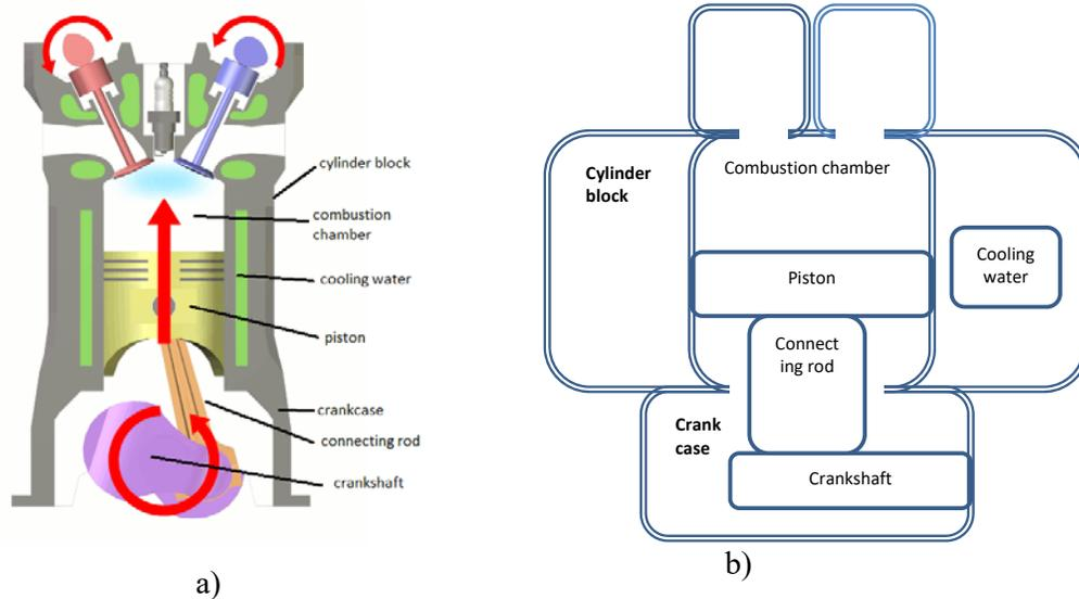
**Figure 1. a) Illustration of a combustion engine<sup>1</sup>; b) Representation of part of the combustion engine with the diagrammatic mereotopological relations.**
