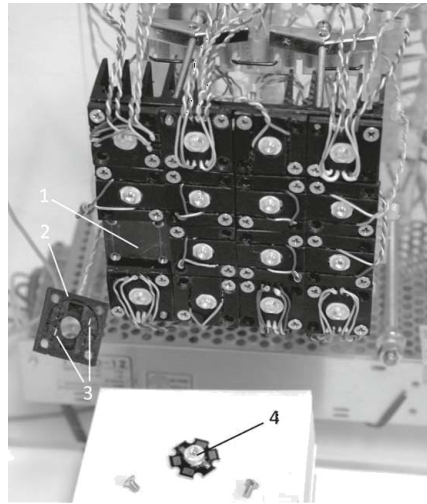
Figure 1: Emitter design: 1 – platform-radiator of MC with LEDs, fixed on it; 2 – plastic clip; 3 – contact pads; 4 – LED, soldered on a standard aluminum board, “star”.
