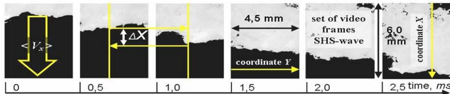
**Fig. 3.** The principle of the interframe difference for determining the velocity of the SHS front coordinates
