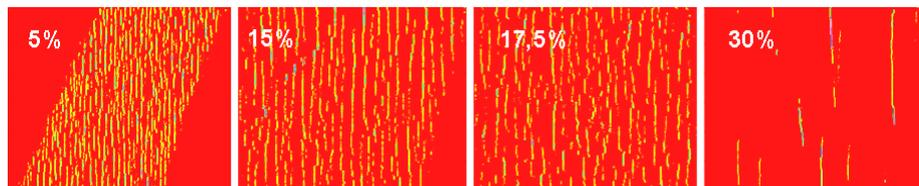
**Fig. 5.** DCS-map of the combustion wave in the Ni-Al system with a change in the proportion of the inert additive
