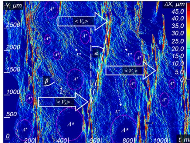
**Fig. 4.** The DCS-map for the heat transfer velocities  $V(x, y) = \Delta X/\Delta t$  in the SHS wave
