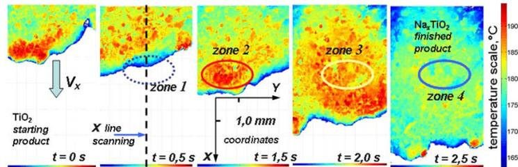
**Fig. 1.** Serial frames of high-speed video (1000 fps) of combustion wave  $\text{TiO}_2$
