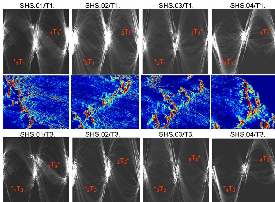
**Fig. 7.** Trace-images: zone SHS.01 – coherent combustion; zone SHS.02 – relay-race combustion; zone SHS.03 – thermal explosion; zone SHS.04 – unstable decay of combustion wave
