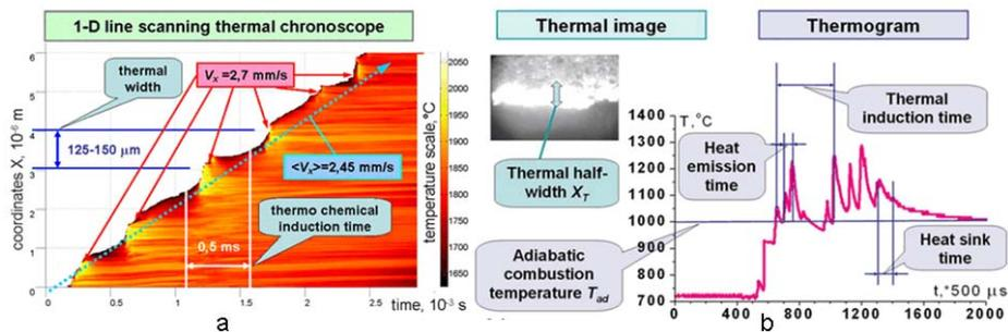
**Fig. 2.** SHT-synthesis of metal oxides: thermogram of the process of solid state burning
