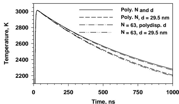
Fig. 1 Relative importance of  $N$  and  $d$  distributions in the flame case:  $T_g = 1720$  K.
