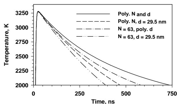
Fig. 2 Relative importance of  $N$  and  $d$  distributions in the low gas temperature case:  $T_g = 440$  K.
