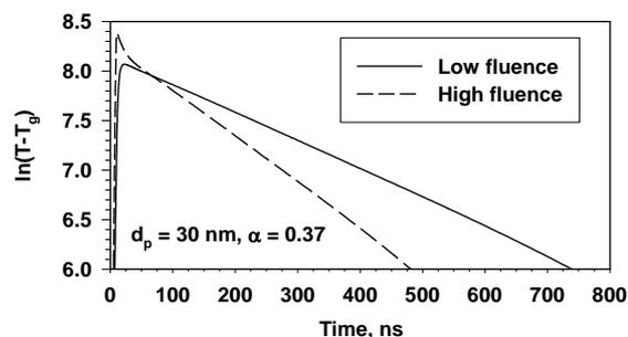
Fig. 3 Particle temperature decay:  $T_g = 300$  K,  $p = 1$  atm.
