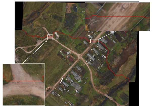
Figure 6: Output mosaic of aerial images with a seam line that bypasses the roads in the optimal way
