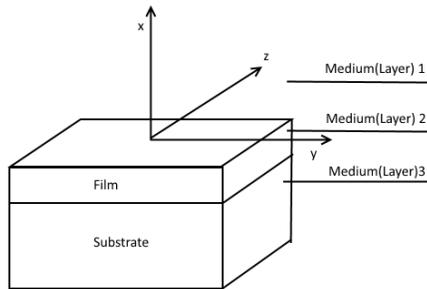
Figure 2. Waveguide is formed by media 1–3
