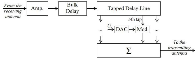
**Fig. 1.** Scheme of the high resolution simulator based on a tapped delay line
