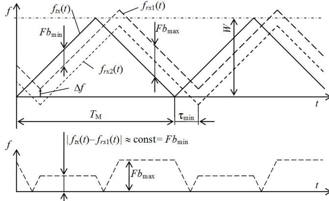
**Fig. 3.** Simulation of the lower altitudes in FMCW altimeters with the triangular modulation
