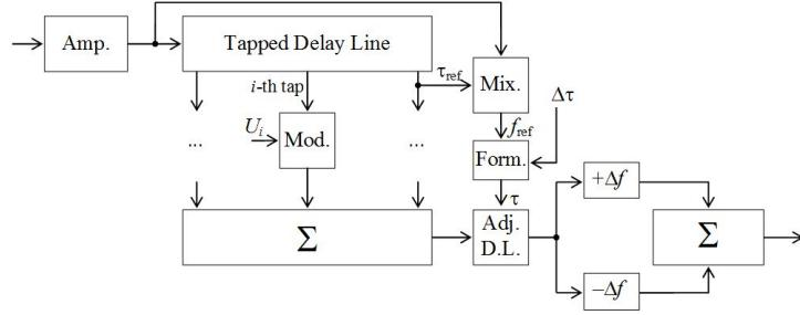
**Fig. 4.** Simulation of lower altitudes for triangular modulation FMCW altimeters
