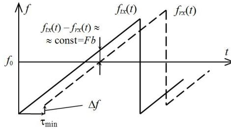
**Fig. 2.** Simulation of an equivalent lower altitude for up-chirp FMCW altimeters
