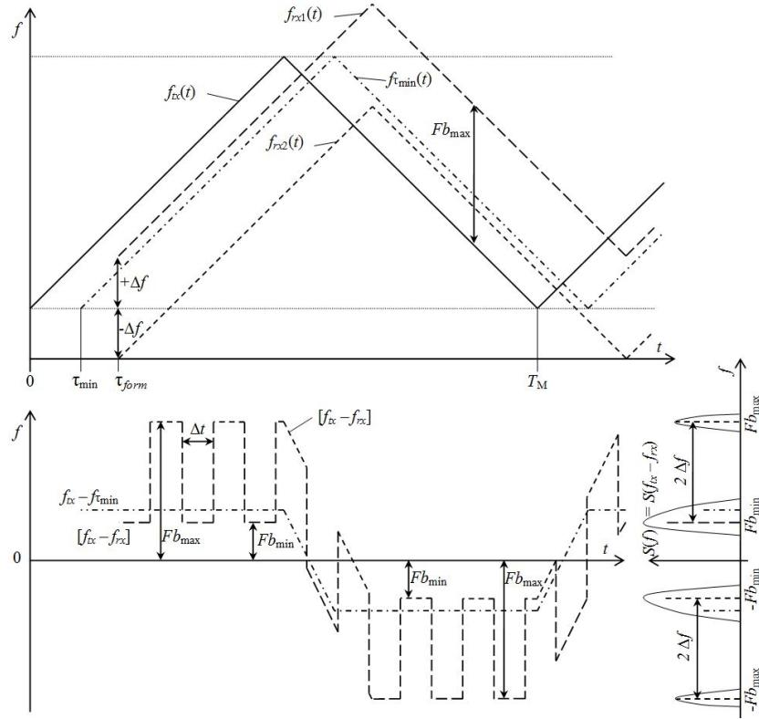
**Fig. 5.** Range harmonics and a beat signal spectrum while simulating the lower distance
