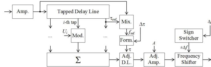
**Fig. 6.** Simulator with the switcher of the sign of the frequency shift
