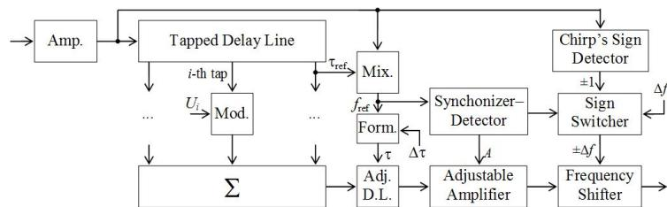
**Fig. 7.** Simulator with the switcher of a sign of the frequency shift
