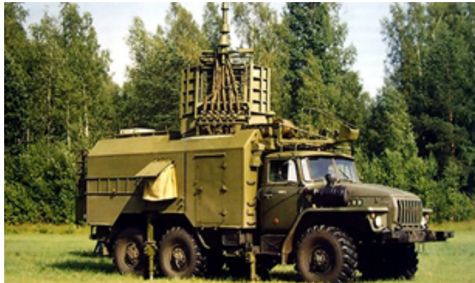
Fig. 8. The station RTR 1L222M “Autobase-M”, maximum range radar reconnaissance — 150 km.
