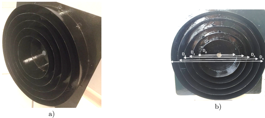
Fig. 5. The system of the five metallic concentric rings (diameters of rings D_0=155 mm, D_1=205 mm, D_2=260 mm, D_3=305 mm, and D_4=355 mm; height H=65 mm; thickness T=1 mm).
