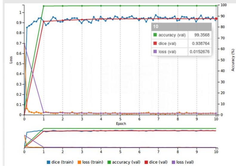
Fig. 4. The result of learning the network FCN-8; dependence of losses and classification accuracy on the number of iterations
