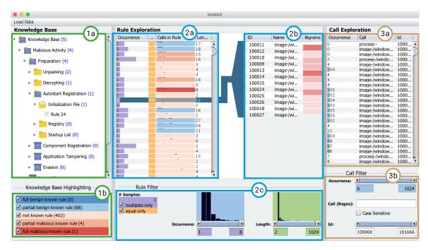
Fig. 1. The BiG2-KAMAS prototype and it's three sections: Section 1 shows the knowledge base including the KDB (1a) with it's new category for benign activity. Beneath the knowledge base highlighting filters are displayed (1b). Section 2 shows the rule exploration area including the bigram visualization (2b) and new color highlighting for benign rules (2a). Finally, section 3 shows the call exploration area.
