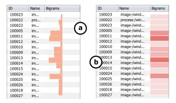
Fig. 2. The two different visualisations methods of the call bi-grams. The first method visualises the bi-grams as bar charts (a), whereas the second visualisation uses the alpha channel to show the severity of the bi-gram (b).
