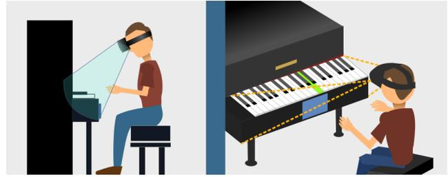
Fig. 1. Illustration of the conceptual design. The user, sitting in front of the piano and wearing an HMD, looks down at the keyboard. When there are notes to be played the respective key is highlighted. Underneath the keyboard there is an image marker which is used for tracking.
