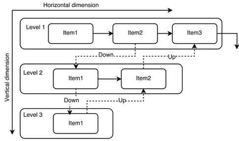
Fig. 1. Horizontal and vertical dimensions or levels. Arrows between items on a horizontal level represent horizontal movement operation. Vertical operations are dashed arrows and labeled.
