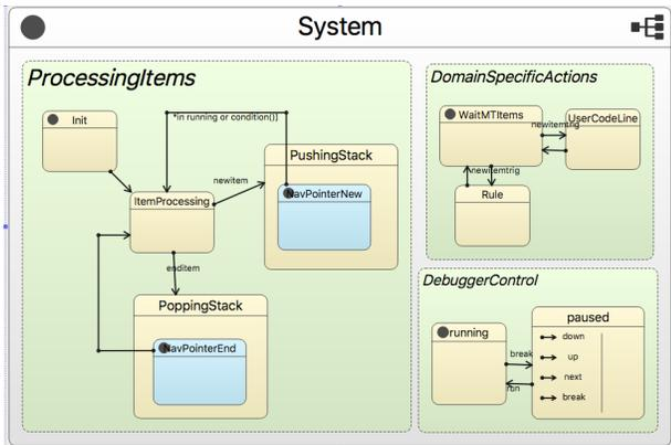
Fig. 5. A *Statecharts* model of the debugger. Orthogonal components are responsible for processing navigation commands, navigation pointers, and implementation specific items corresponding to navigation pointers.
