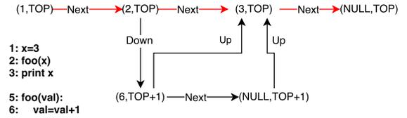
Fig. 2. Navigation pointer evolution. Red arrows represent a step-over debugging scenario.
