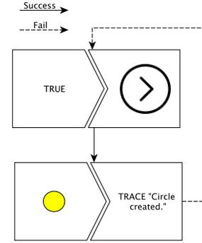
Fig. 4. A debugging scenario that steps through the MT execution until the circle pattern is found resulting in a trace message.
