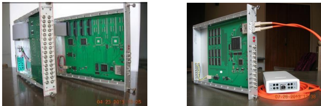
Figure1. In the photo on the left is an MPD board, on the right is a De-Li-DAQ-2D module
