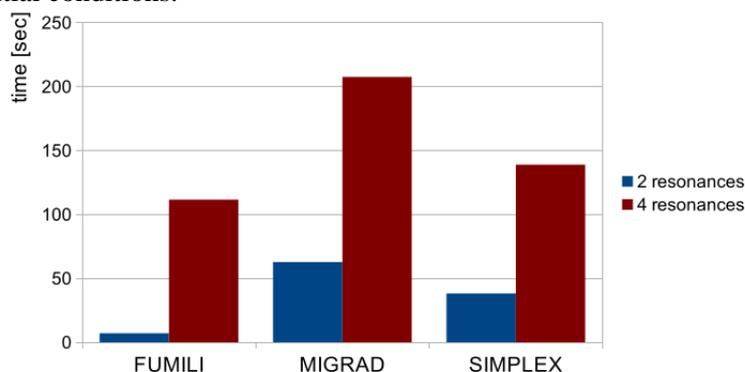
Figure 1. Convergence time for the different minimization methods
