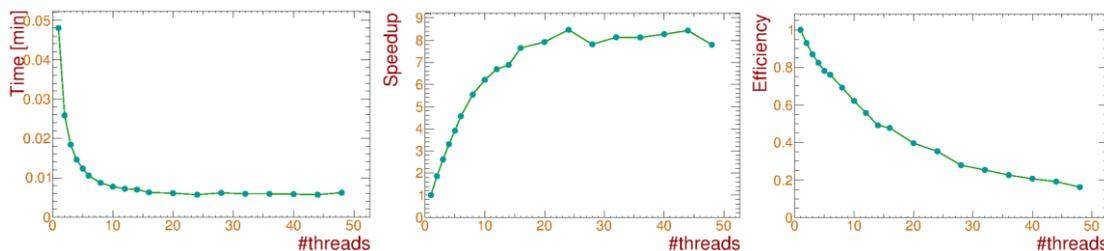
Figure 3. CPU benchmarks: time, speedup, efficiency (2 Intel Xeon E5-2695v2 CPUs)
