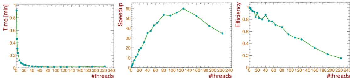
Figure 4. Co-processor benchmarks: time, speedup, efficiency (Intel Xeon Phi 5110P)
