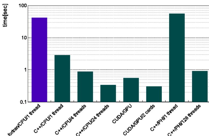
Figure 2. Average call time for test function with gradients, 5 resonances
