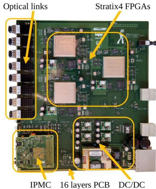
Figure 6. Picture of the ABBA board
