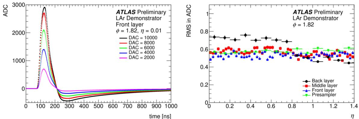
Figure 7. LAr demonstrator calibration pulse shapes for a front layer super cell at  $\phi = 1.82$  and  $\eta = 0.01$  for different input DAC values (left) and noise level of super cells in ADC counts for different layers (right) [6]
