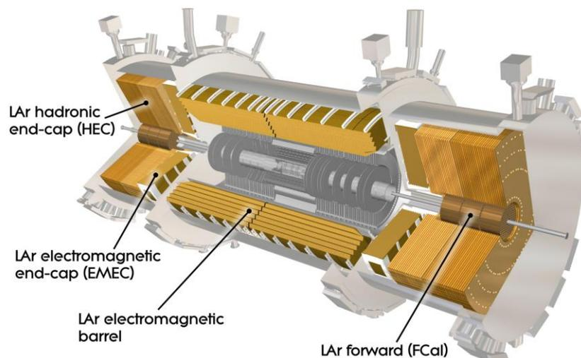
Figure 1. The scheme of the ATLAS LAr Calorimeter (ATLAS Experiment © 2008 CERN)
