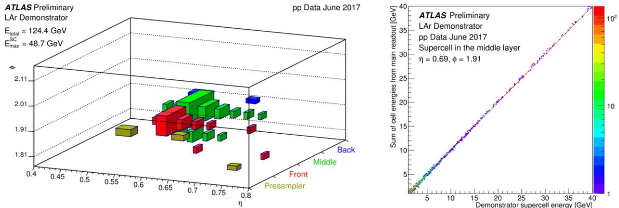
Figure 8. LAr demonstrator proton-proton collision data: Event display of the partial demonstrator region with a total energy of 124.4 GeV (left) and correlation of energy measurements for one super cell at  $\phi = 1.91$  and  $\eta = 0.69$  in the middle layer (right) [6]
