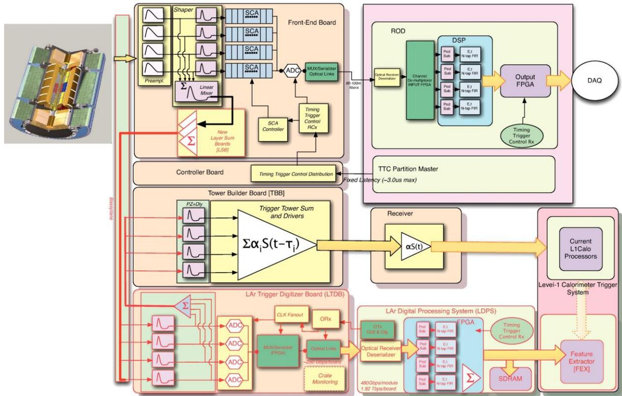
Figure 4. Schematic block diagram of the Phase-1 upgrade LAr trigger readout architecture. The new components are indicated by the red outlines and arrows [3]
