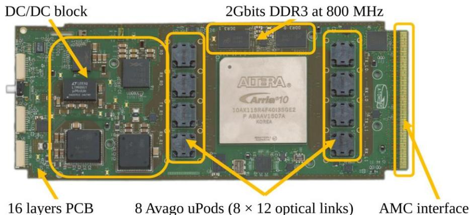
Figure 5. Picture of the LATOME board
