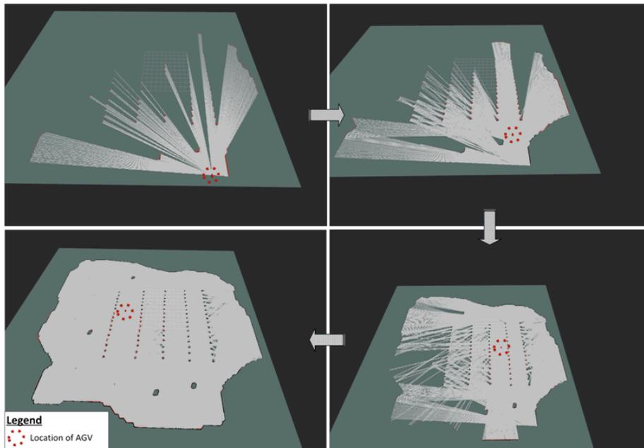
**Fig. 4.** Inflated layout with ROS global and local path generation.
