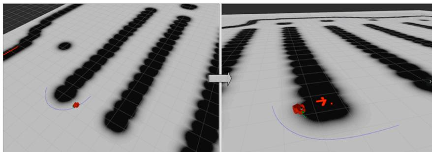
Fig. 3. Inflated layout with ROS global and local path generation.
