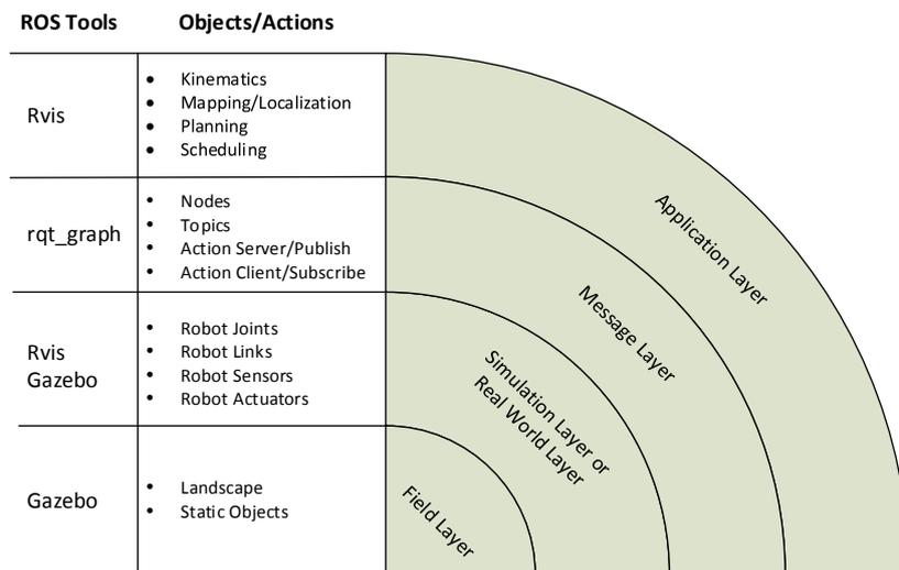
**Fig. 1.** Overview of the system components and related inter-connections.
