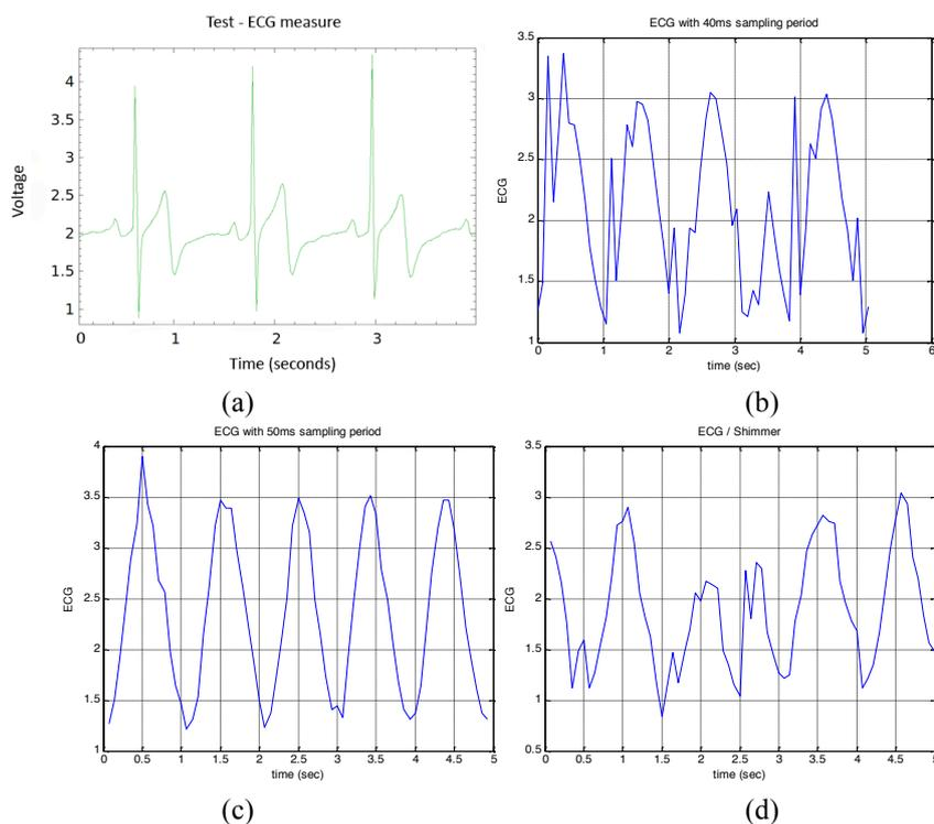
**Fig. 4.** Reference Cooking Hacks e-Health ECG sensor output (a), real ECG output using a sampling period of 40ms (b), 50ms (c) and Shimmer ECG output (d).
