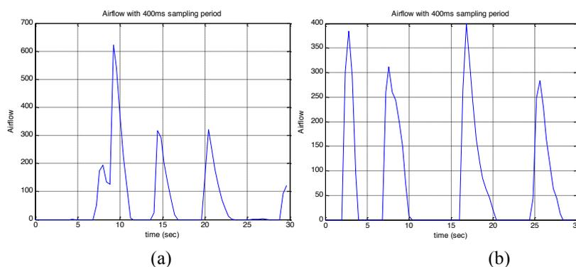
**Fig. 2.** Breathing patterns applied to the airflow sensor: a deep breath followed by two shallow ones (a) and two pairs of deep/shallow breaths (b).
