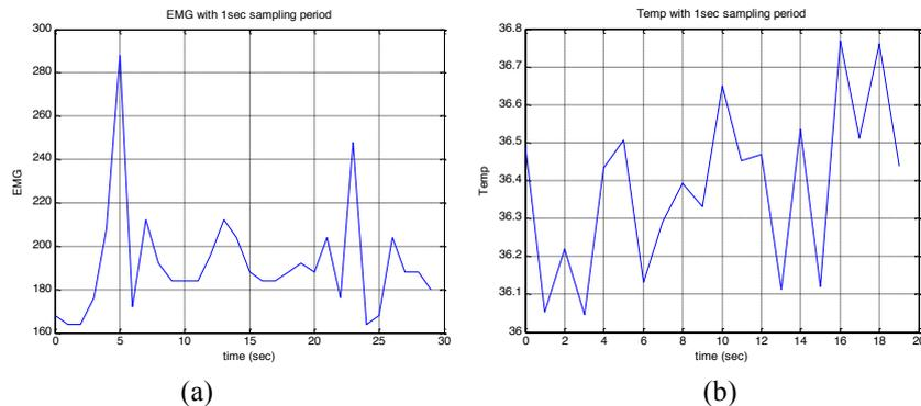
**Fig. 3.** EMG sensor output for two strong muscle contractions and three less strong muscle contractions in between (a). Temperature sensor output for a person that has a temperature of 36.5 °C (b).
