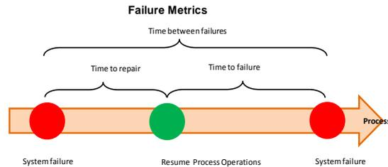
Fig. 3 Failure milestones.
