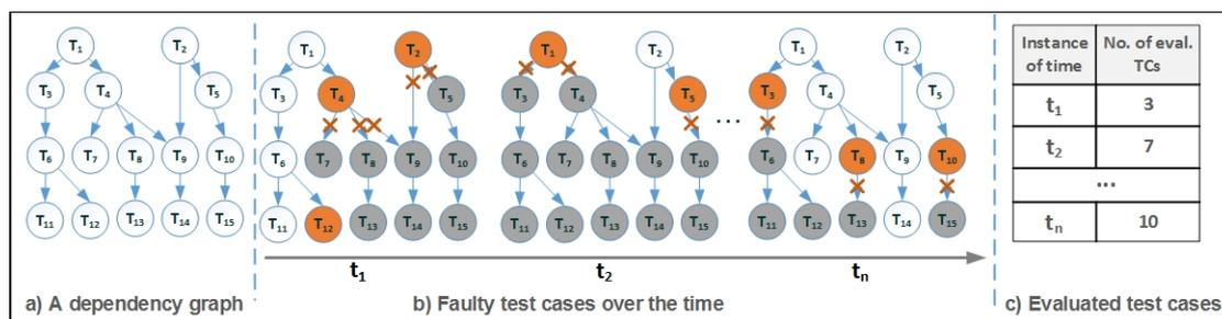
**Figure 3.** The *EffTE* Approach. (a) A test case dependency graph; (b) faulty test cases over time (orange nodes are faulty test cases), gray nodes represent test cases ignored for evaluation; and (c) number of evaluated test cases (TCs) per instance of time. Dependencies enable to ignore faulty test cases.
