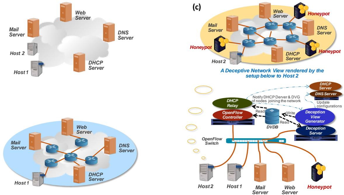
Figure 1. ACyDS enables rendering of different network views to hosts on the same physical network
