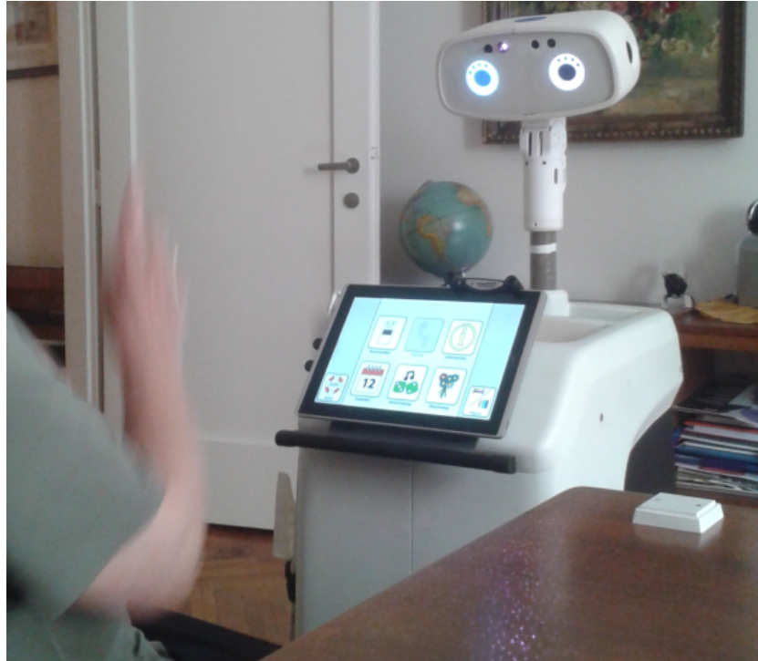
Fig. 1. The Hobbit robot facing a user. The active head is used to clearly indicate to the user when the robot expects input. On the right side of the body a part of the gripper and robot arm is visible. On the table is a battery-less call button to initiate interaction with the robot.
