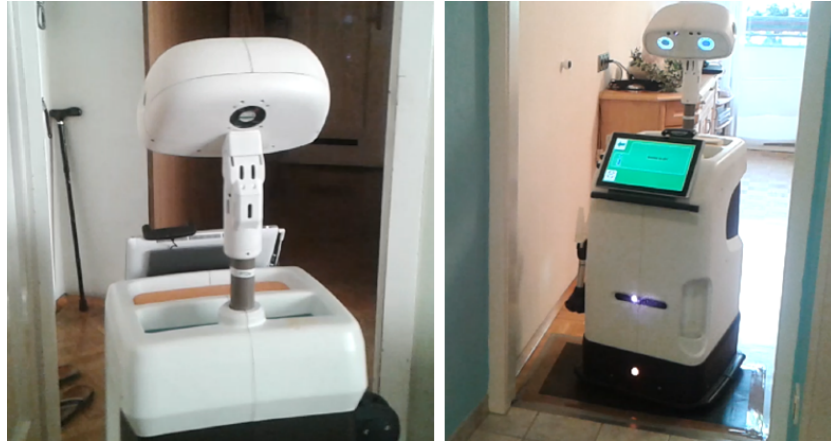
Fig. 3. Two example of narrow doors of 0.7 m in homes of two Swedish users. The robot is 0.56 m wide and should be slimmer.
