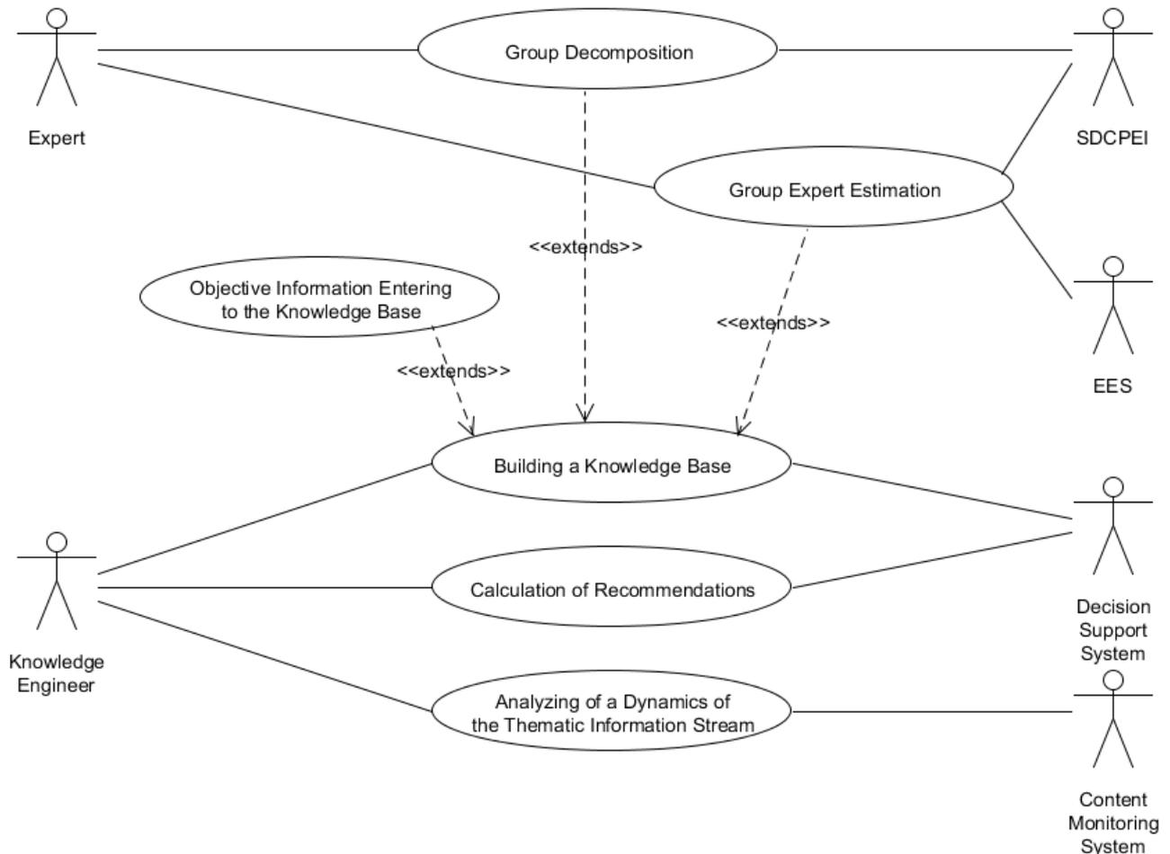
Fig. 10. Use Case Diagram of the Concept of Information-analytical System for Information Operations Detection
