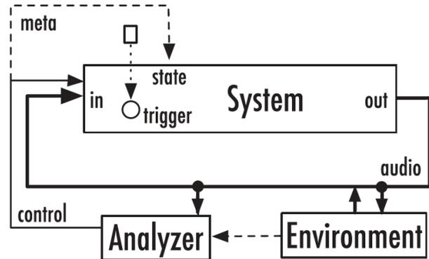
Figure 2. A general scheme of feedback systems according to Sanfilippo and Valle [17].
