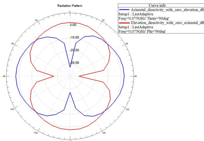
**Fig. 3.** Azimuth plane (blue line) and elevation plane (red line) radiation patterns
