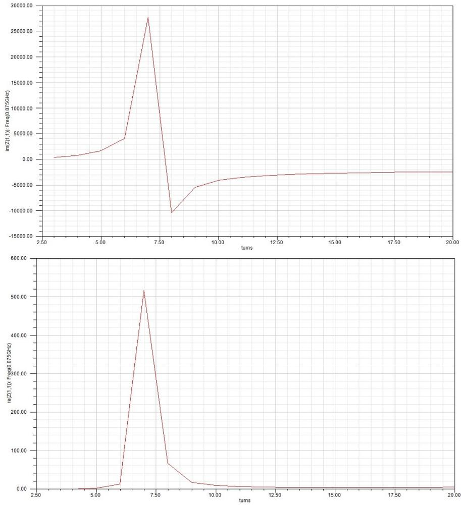
**Fig. 4.** Parasite resonance, depending on the number of wire turns at fixed frequency 75MHz: imaginary (above) and real (bottom) components of the antenna input impedance
