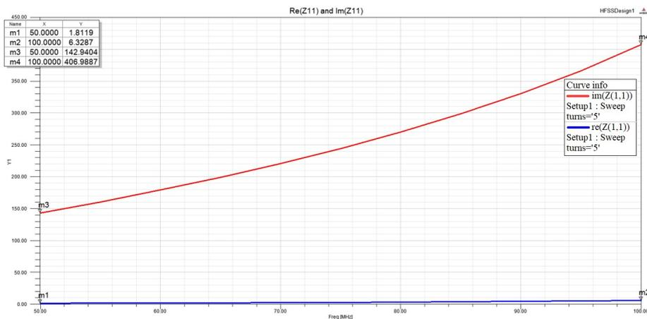
**Fig. 2.** Antenna input impedance: imaginary (red line) and real (blue line) parts
