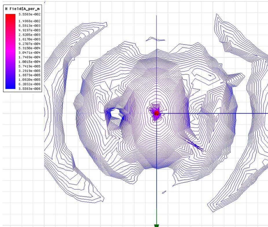
Fig. 8. Magnetic field intensity in the near-field zone, A/m
