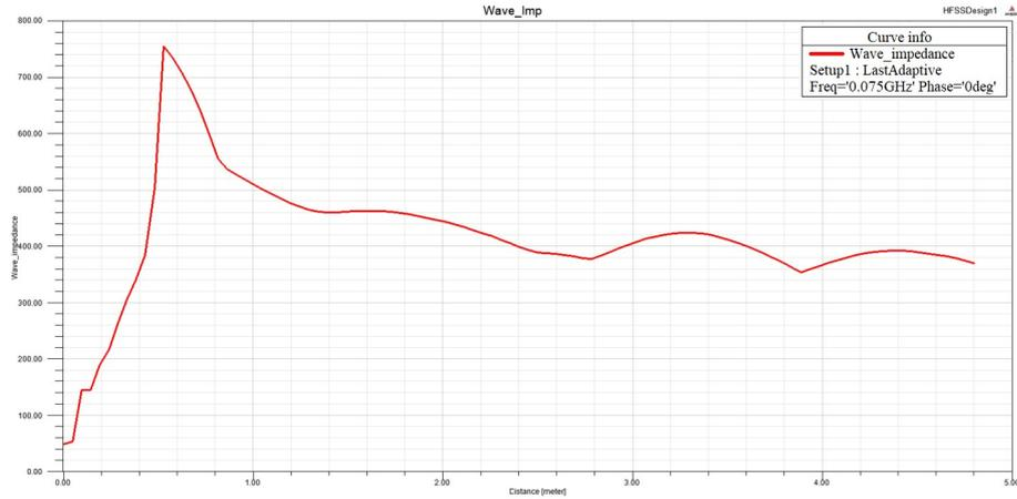
**Fig. 6.** Estimation of the far-field radiation boundary by wave impedance, Ohm
