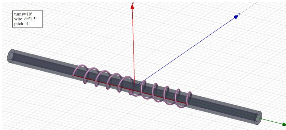
**Fig. 1.** 3D-view of a ferrite antenna model
