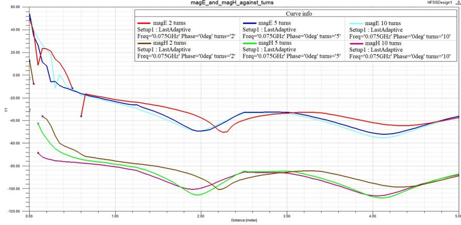
**Fig. 5.** Intensities of the electric (upper curves) and magnetic (lower curves) fields depending on the number of wire turns, dB
