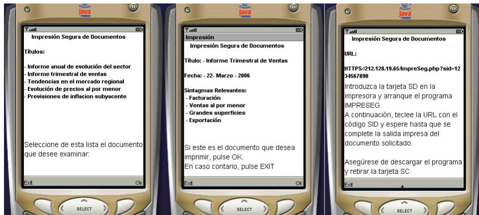
Fig. 1. Example on a dialog for a document secure printing. In the search phase, the titles of candidate documents are shown. In the identification phase, it is shown the metadata associated with a document and, in case of a positive identification, the server provides an URL with a session identifier which allows to request the document printing from a multifunction printer.
