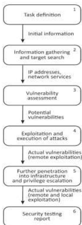
Fig. 1. Security testing flow chart
