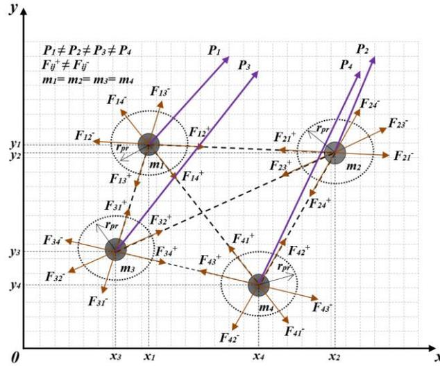
**Fig. 4.** The scheme of forces with four dynamic objects in the original position
