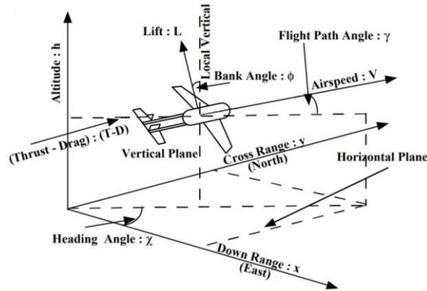
**Fig. 2.** UAV coordinate system
