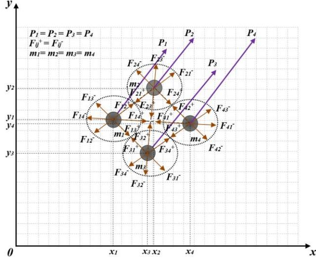
**Fig. 5.** The scheme of forces with four dynamic objects after group formation
