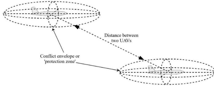
**Fig. 3.** Spheroidal conflict envelope or ‘protection zone’ and distance between two UAVs in the vertical plane
