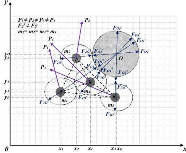
**Fig. 6.** The scheme of forces with four dynamic objects in a group avoiding an obstacle
