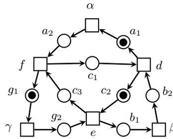
**Fig. 4.** Net System representation for the Transition System in Figure 1, the marking corresponds to state 1
