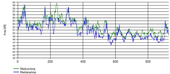
Figure 7. Statistical median and simple average for a shorter time slice. Windows size is set to 20.
