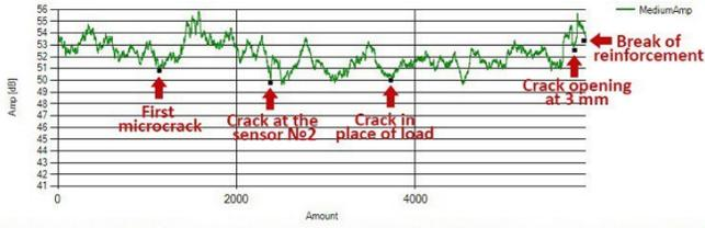
Figure 8. Simple moving average for different stages of beam destruction. X-axis indicates the number of signals, Y-axis indicates amplitude.
