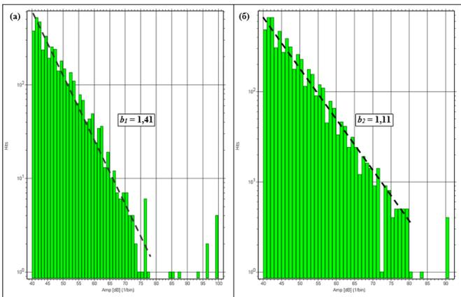
Figure 9. Plots of amplitude distributions for different stages of beam destruction and their  $b$ -values
