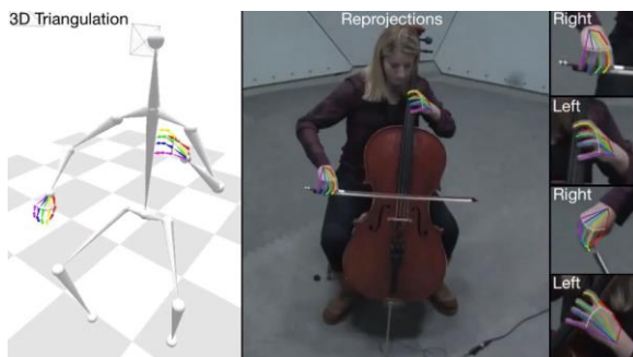
Figure 9 - Hand pose estimation generated by RGB data from different viewpoints 6
