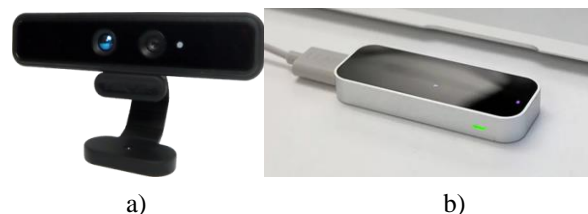
Figure 7 - a) DepthSense DS3252 2 and b) Leap Motion sensor 3 .
