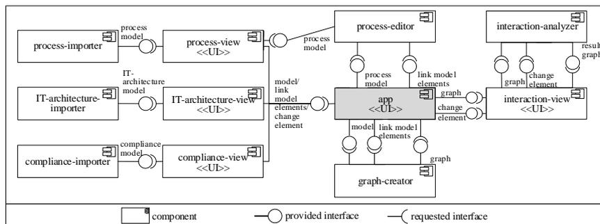
**Fig. 2.** BCIT architecture as a UML component diagram
