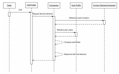
Figure 2: Interactions with the Call Profiler Service
