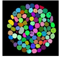
**Figure 10.** Slice of segmented 3D image with proper segmentation; parameters according to maximal Q were selected.
