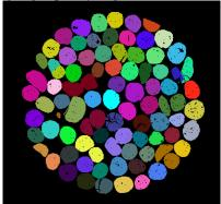
**Figure 9.** Slice of segmented 3D image with several separated and merged particles; fixed parameters were used for segmentation.
