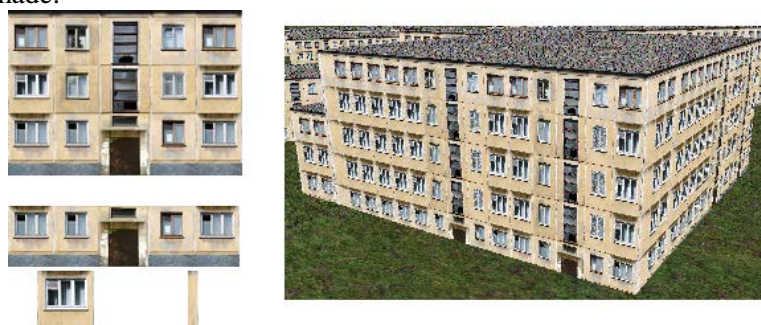
Figure 6. Standard texture for the building wall; division of the texture into sections: the entrance, the window, the wall and the resulting 3D model.
