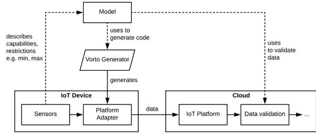
Figure 1: Using VortoFlow in an IoT pipeline.
