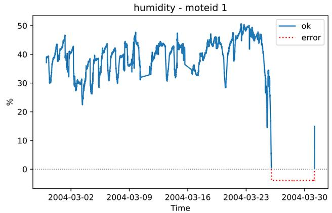
Figure 3: Errors in humidity readings (Mote with id 1).
