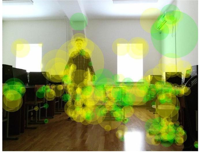
Figure 5: Example of features matching on the RGB image with the human being
