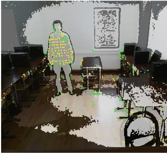
Figure 4: Example of features matching on the RGBD image (RGB+DepthMap) with the human being
