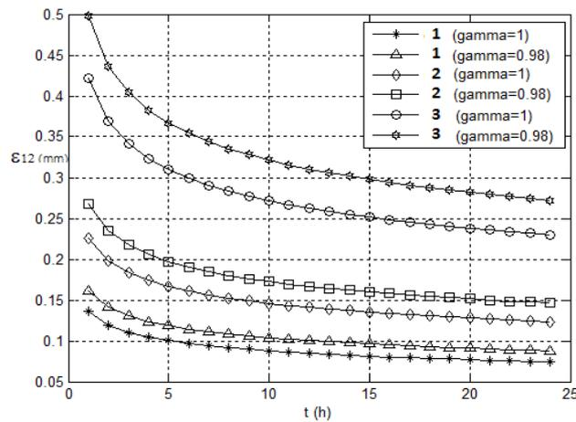
**Fig. 3.** Change in the deformation component  $\varepsilon_{12}$  depending on the type of biomaterial
