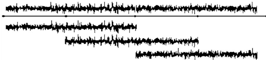
**Fig. 3.** Illustration of segmentation by Welch's method. For each segment, periodogram is estimated and obtained periodograms are averaged.
