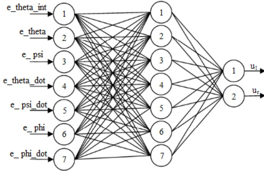
**Figure 4.** Neural network controller structure.
