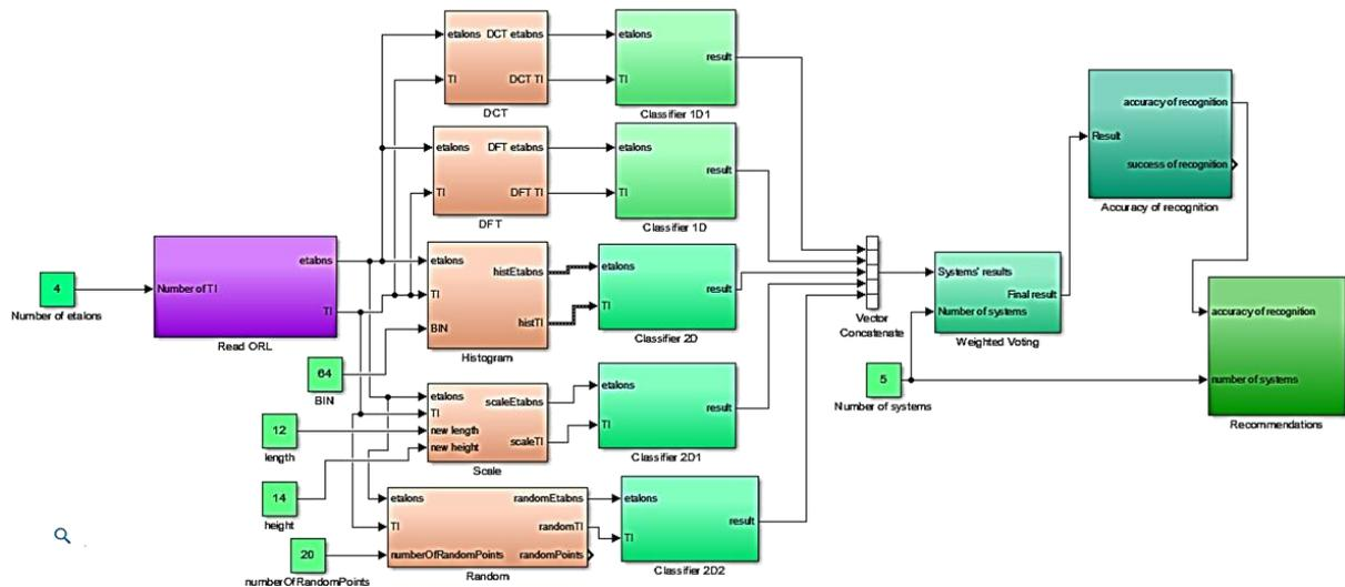
Figure 4. Example of parallel facial image processing systems
