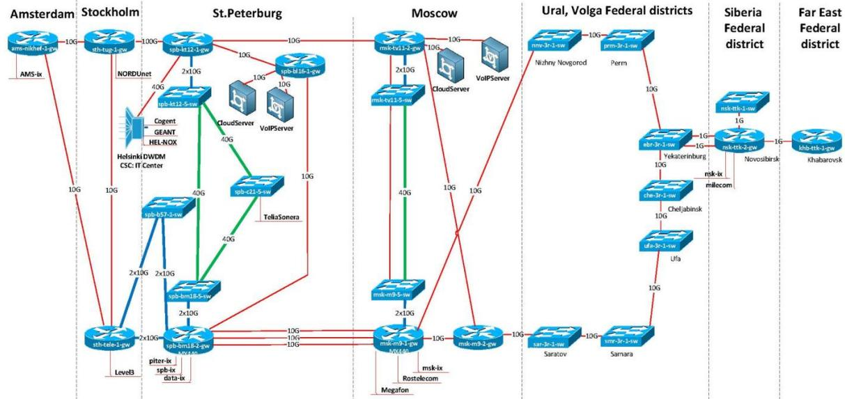
Figure 1. High-Level Design network architecture of the RUNNet network
