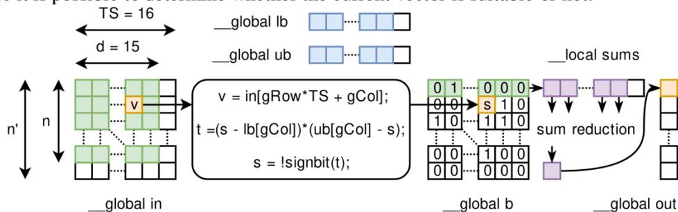
Figure 3. The structure of the OpenCL procedure GPU2 for parallel data processing
