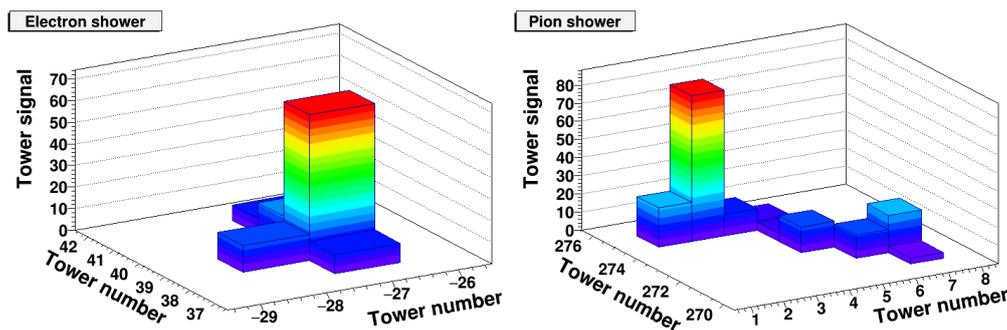
Figure 4: Left - ECal tower signal distribution obtained for a 0.5 GeV/c electron; right – the same for a 0.5 GeV/c pion. Horizontal axes represent the tower numbers in the longitudinal and tangential directions with respect to the beam line. Vertical axis shows the signal amplitude.
