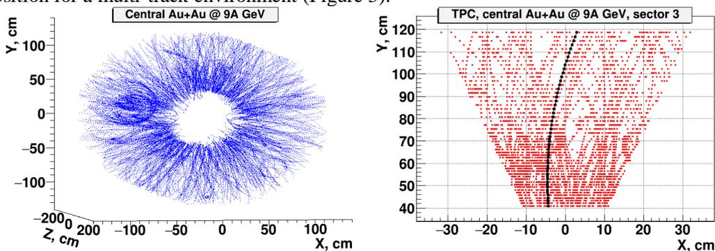
Figure 2: Left - 3-D visualization of trajectories of charged particles in the TPC, produced in Au+Au collision at  $\sqrt{s_{NN}} = 9$  GeV. Right - transverse projection of particle trajectories passing through one readout chamber. Dots represent particle crossing points with median planes of pad rows. Black line shows a track of a 0.5 GeV/c pion.
