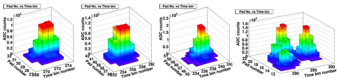
Figure 3: Left - charge distributions from 3 pad rows obtained for a 0.5 GeV/c pion from Figure 2 in the pad number versus time bin space. Vertical axis represent the signal amplitude. Right - charge distribution from several close tracks.
