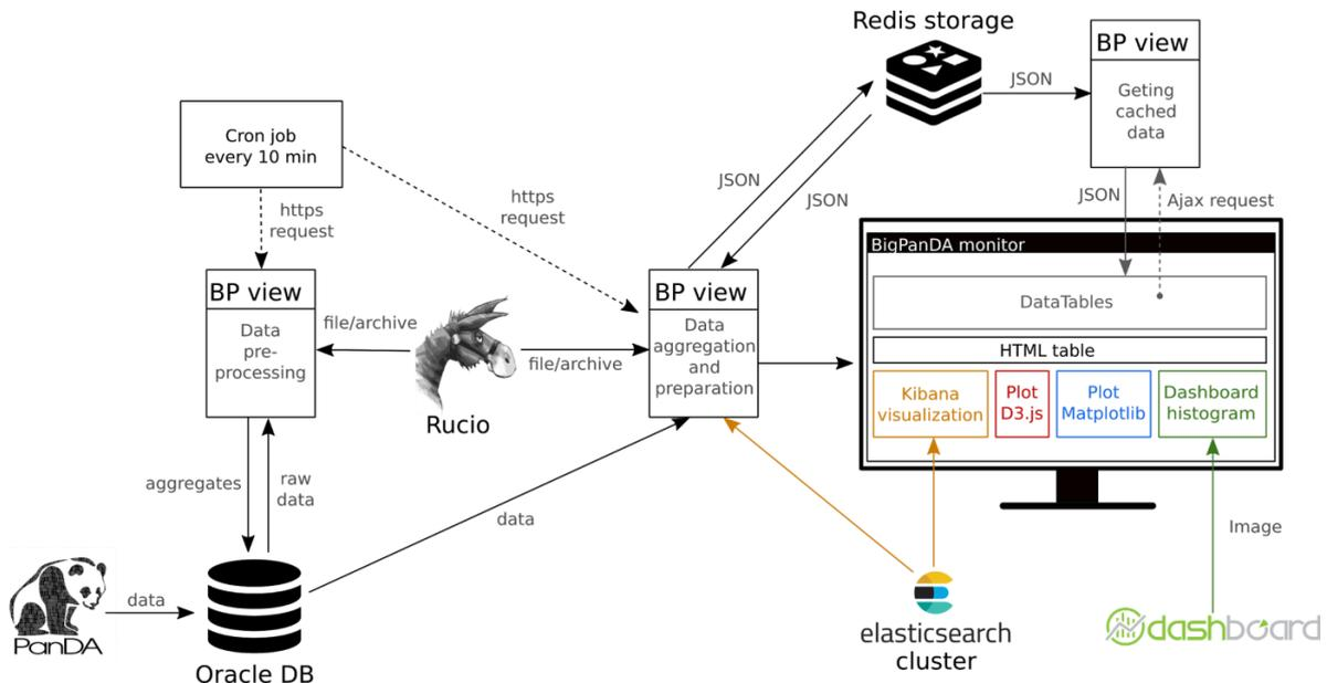
Figure 2. Data-flow diagram of the BigPanDA monitor
