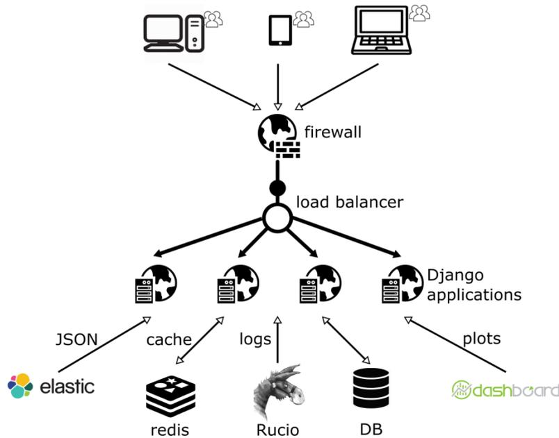
Figure 1. Architecture scheme of the BigPanDA monitor instance
