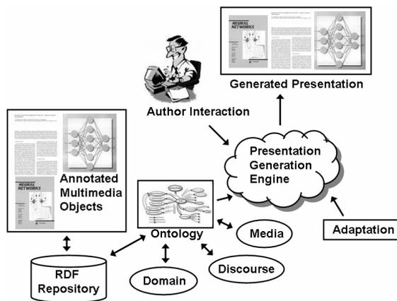
Fig.3. Logical diagram of the system
