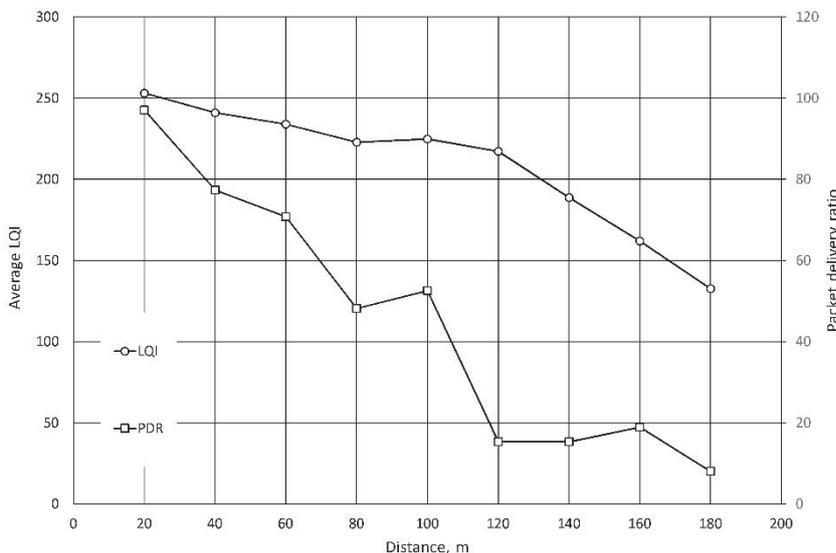
Fig.5. Influence of the distance between nodes on measured average LQI and PDR for outdoor
