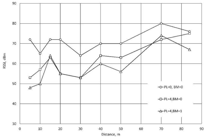
Fig.3. Influence of the distance between nodes on measured average RSSI value for indoor
