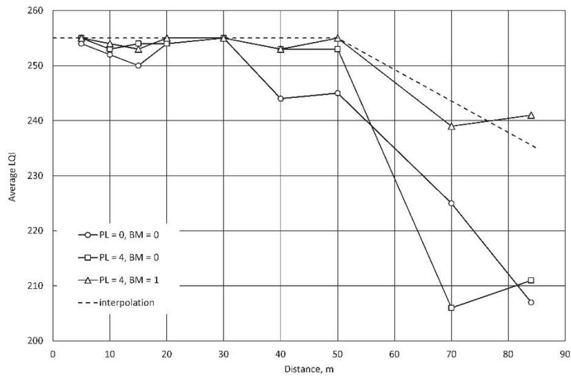
Fig.4. Influence of the distance between nodes on measured average LQI value for indoor
