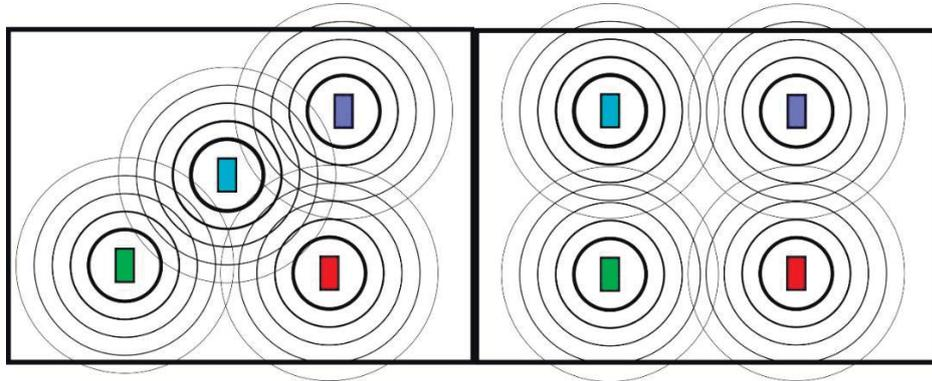
Fig.1. Examples of sensor nodes deployment in closed field (a – non-optimal deployment, b – optimal deployment)
