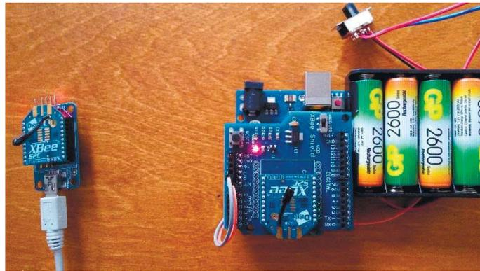
Fig.2. Experimental setup for LQI measurement
