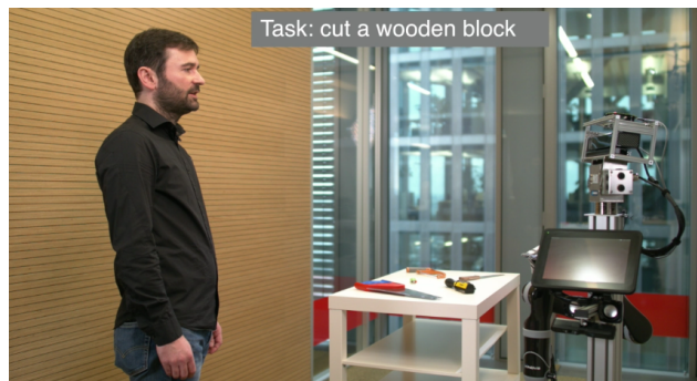
Figure 1: Illustration of the scenario. The robot IRA and the user are in a room. The user can ask IRA how to manipulate an object. IRA explores the table, detects the tools and proposes a suitable tool via speech.
